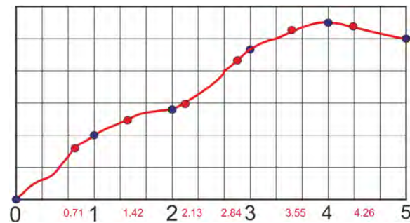
Figure 3: Interpolation with floating nodal points
